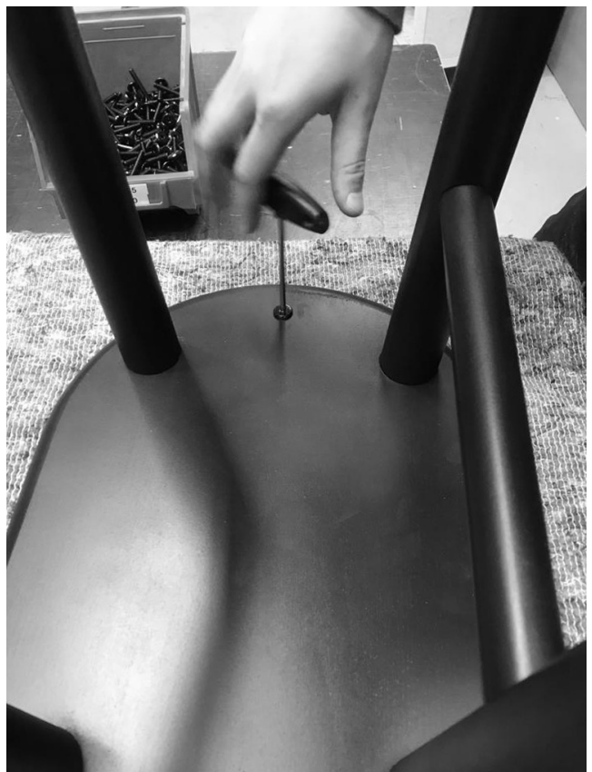
mount the pads on the seat with the bolts
