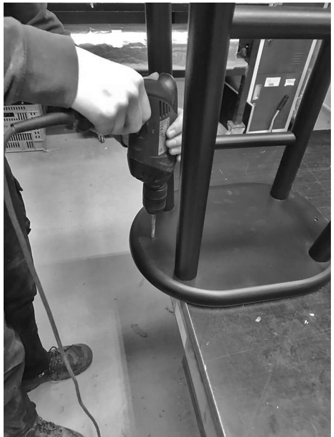
drill through with a 6 mm wood drill
